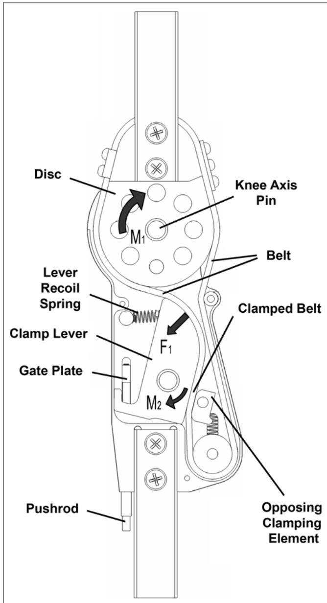
**Figure 6.** Friction-based Ottawalk belt-clamping knee joint in stance mode with applied flexion moment.  $F_1$  = belt force on clamp lever,  $M_1$  = knee moment,  $M_2$  = clamp lever moment.
