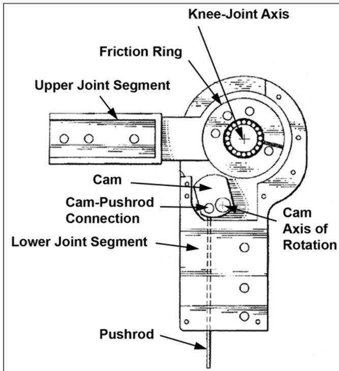
**Figure 3.** Cross-sectional view of Horton Stance Control Orthosis locking mechanism—unlocked and in 90° knee flexion. Hatton BJ, Hatton DL, Wallace ZG. 2003. Articulating knee supports. United States patent US 6635024. 2003 Oct 21.
