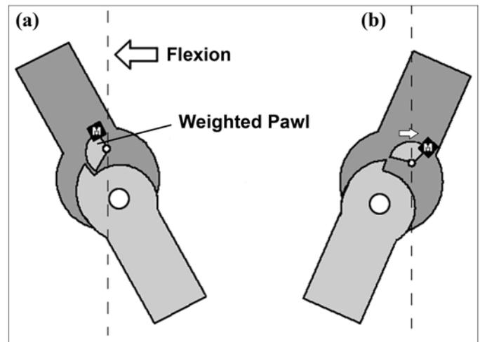
**Figure 4.** Gravity-activated Fillauer Swing Phase Lock with pawl weighted by mass ( $M$ ): (a) when thigh is anterior to user's body and knee is fully extended, weighted pawl falls into locked position; (b) with thigh posterior to user's body and knee extension moment, pawl falls out of engagement.
